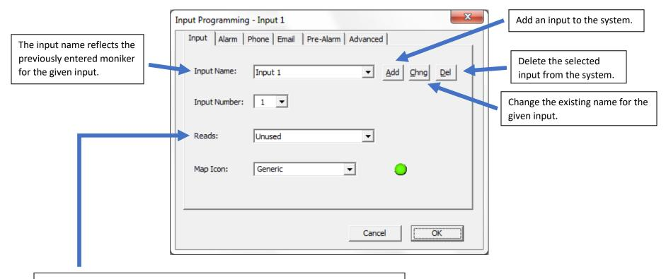
In order to set up a given input you must correctly identify and select how that input is identified by the system. By clicking on Reads you can set the type of probe that is being read, the value of measurement for that probe, the scalar parameters for a linear transducer, and the ability to make an input a type of switch contact.
